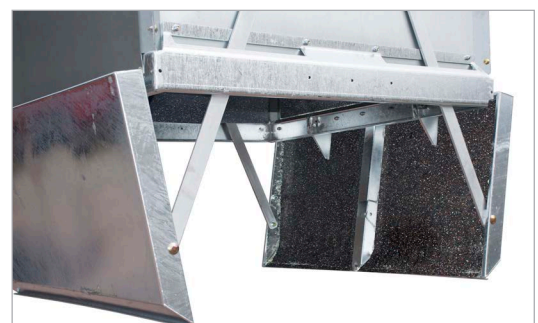
Collecting of glass: chains, trap doors and bottom section of walls (up to 1 m) with noise insulation
